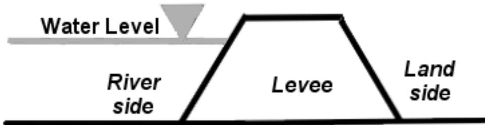
**Levee is not overtopped and is not breached.**
