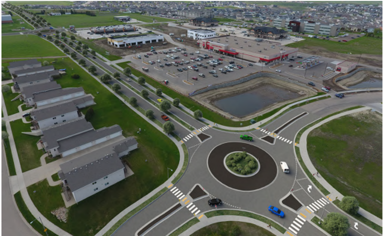
Alternative B: Three-Lane Section with Roundabout Intersections
