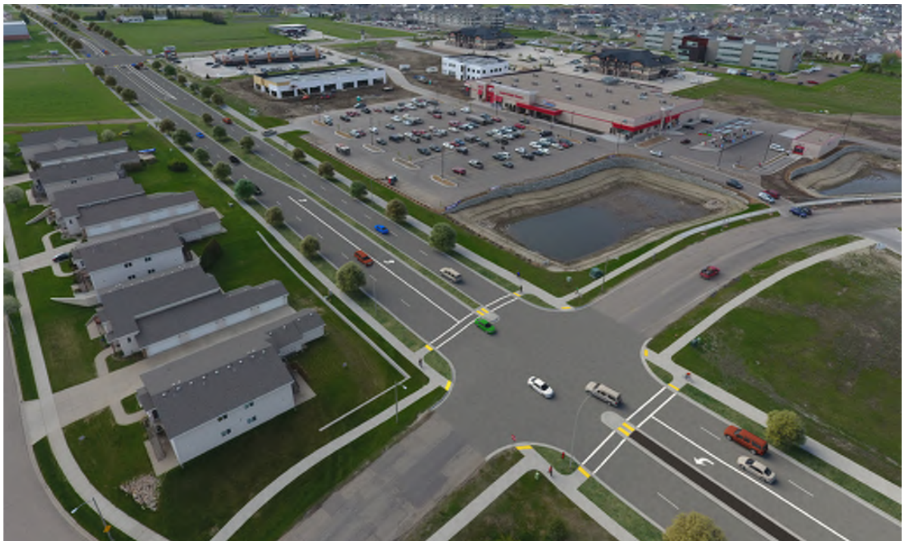
Alternative C: Five-Lane Section with Future Signalization
